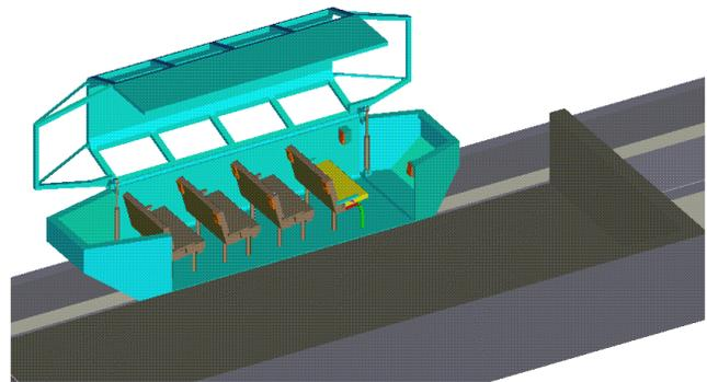
The guideway is a single box beam with a slot at the top. The wheel set is entirely inside the box beam.
