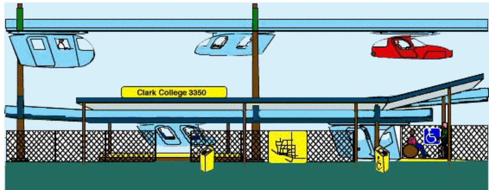
There are several models of vehicles in development; only the Dove (standard, 2 passengers) and Pelican (wheelchair accessible, 1 passenger) vehicles are mentioned in this report. Specially made dual mode cars and cargo carriers are also in design. The Dove has two seats, one in front of the other (tandem seating). Each rider has a separate door and automatic safety restraints.
