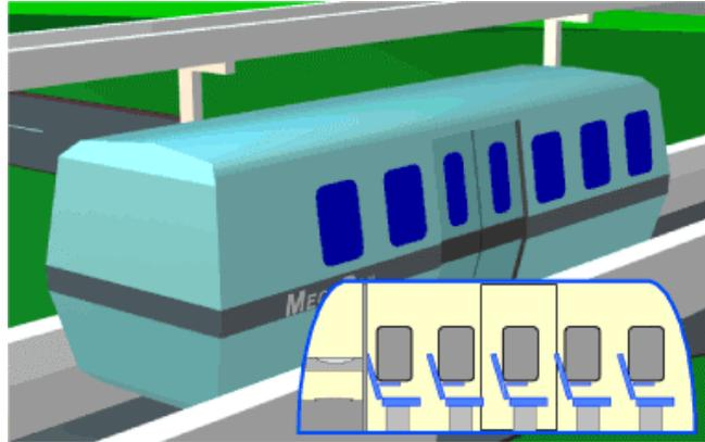
A small-scale operating car was built and successfully tested to validate the vehicle steering and switching approach. Detailed engineering drawings for the vehicle, rail and guideway have been prepared. A 1/5-scale prototype is now being built. In addition to the small-scale models, a full-size section of MicroRail guideway has been fabricated, erected, and static load tested.
